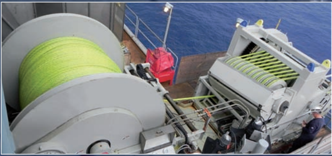
The 80t capacity Perdido synthetic traction winch with 3300m of 60mm Samson Quantum-12 rope.
